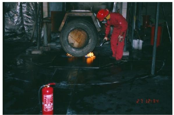
Figure C.5: Ignition of the hepthane soaked rags under the tyres.
