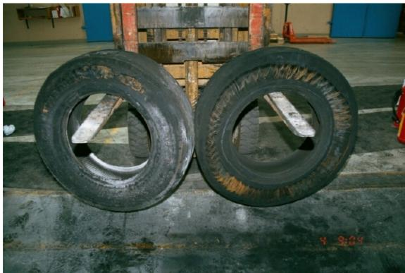
Figure C.12: Two tyres after a tyre fire trial.
