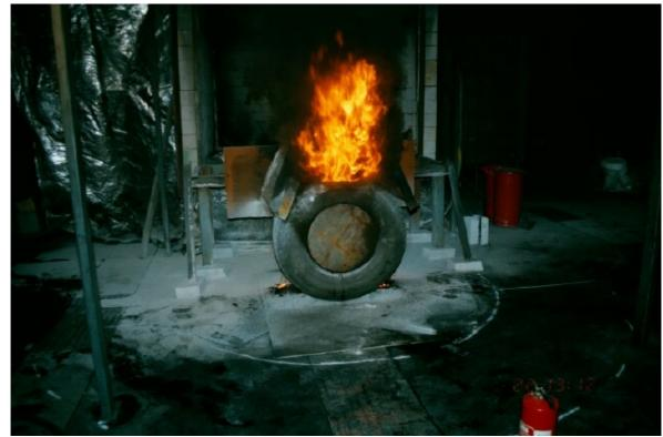
Figure C.6: In the early phase of the tyre fire.
