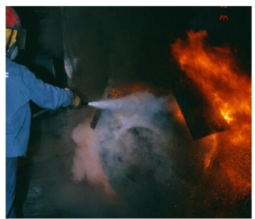
*Figure C.8: The start of fire fighting with a dry powder fire extinguisher.*
