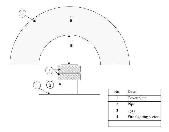
Figure 2.2: A sketch showing the marked area in which the fire fighter was allowed to move within on the floor in front of the tyre.
