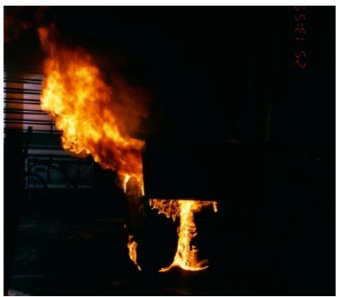
Figure C.7: The state of the tyre fire when the heat release rate approaches 500 kW and it is immediately before fire fighting starts.
