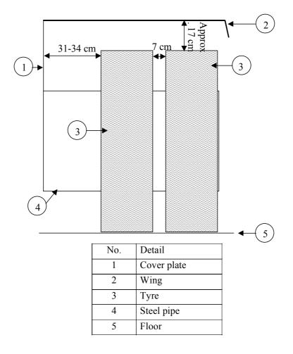
Figure 2.1: The test arrangement used for the testing of the efficiency of different fire extinguishers against twin tyre fires.
