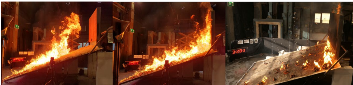
Figure 2-11: Fire spread in the experimental set-up with an inclined fuel bed and untreated wooden materials. Note that the cavity behind the cladding caught fire and had to be extinguished. (Photo: RISE Fire Research/TREADS).
