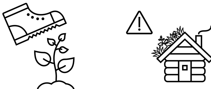
Figure 3-2: Left: Stomping on the heather on the ground around a cabin makes the ground more compact, which is beneficial to prevent fire spread to the structure. Right: Many structures in Norway has vegetation on the roof, and it is important to keep this short and alive to minimize the ignition hazard.
