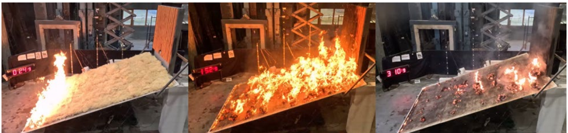
Figure 2-12: Fire spread in the experimental set-up with an inclined fuel bed and treated wooden materials. Note that the cavity behind the cladding did not catch fire. (Photo: RISE Fire Research/TREADS).
