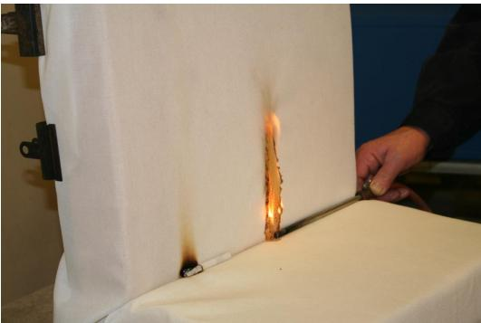
Figure 7-2Demonstration – smouldering cigarette and match-flame equivalent on an<br/>IMO 2010 FTPC Part 8 upholstery material assembly.
