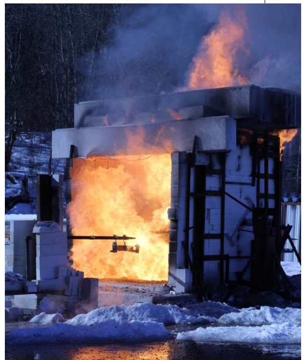
Jet fire testing of cryogenic spill protection. The test specimen is subjected to cryogenic cooling (upper image), directly followed by a jet fire test (lower image).
